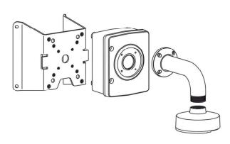
The corner mount adapter allows easy installation to the corner of a building. With the adapter fitted, a wall mount and surveillance cabinet can be added to provide a full weatherproof installation option.
