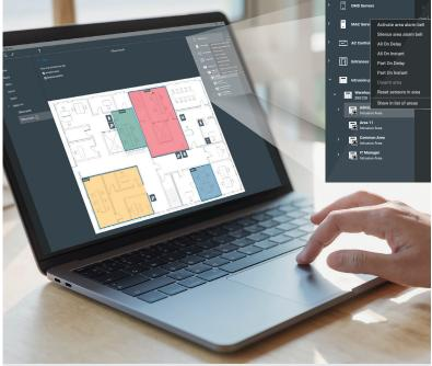
The interactive map allows you to control intrusion panels. Multiple map levels allow you to see your entire enterprise or focus down to one particular door or area.
